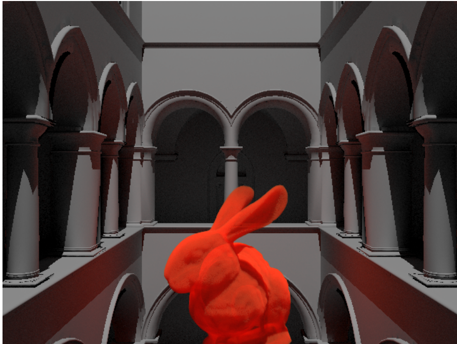
Figure 6.1: The Sponza Atrium with the Stanford volumetric bunny. In-/Out-scattering is evident on the volume and on the surrounding atrium walls.
