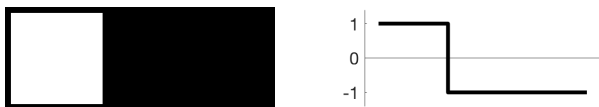
Fig. 3: Haar-like feature kernel (left) and a horizontal cross-section of the kernel (right)
