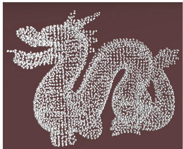
Figure 2: A ray traced rendering of the dragon model with approximately five thousand spheres.
